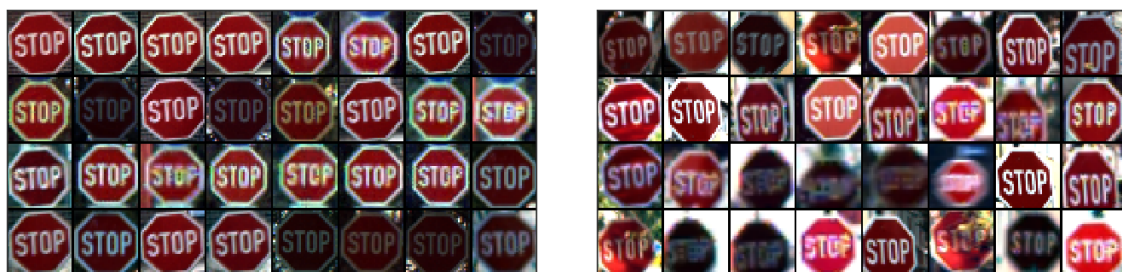
Figure 6: Example from one experiment (seed) of the 32 most normal (left) and 32 most anomalous (right) examples on GTSRB stop signs training set according to Deep SVDD anomaly scores ordered by score from top left to bottom right.
